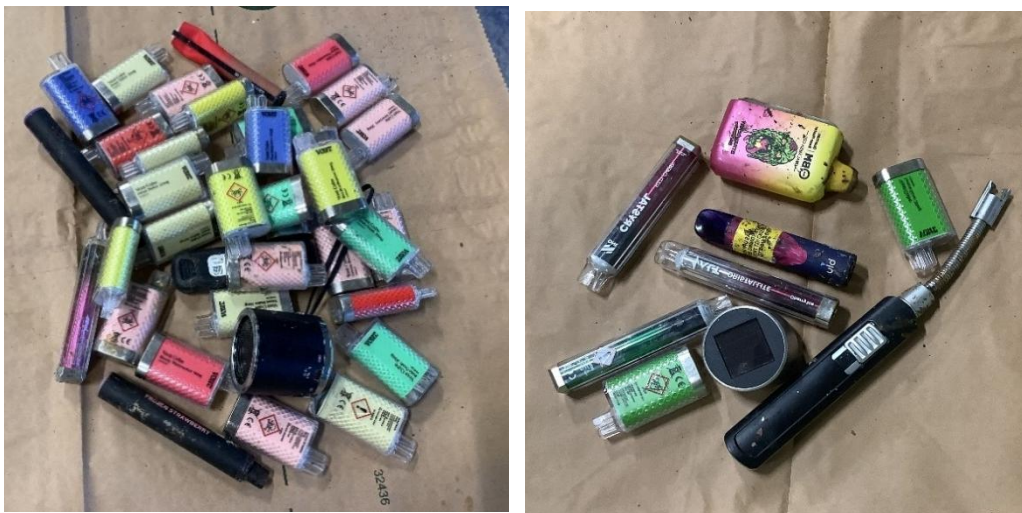
Figure 1. Pictures of the fraction "WEEE with embedded batteries" from the complementary waste composition analyses. Photographer: staff at Envir.
