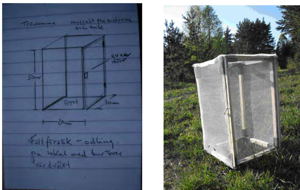
Figure 3. Drawing of the construction scheme by Göran Palmqvist (spring 2007) and photo of a cage at the flight area near Lojsta Russpark (May 2007).
