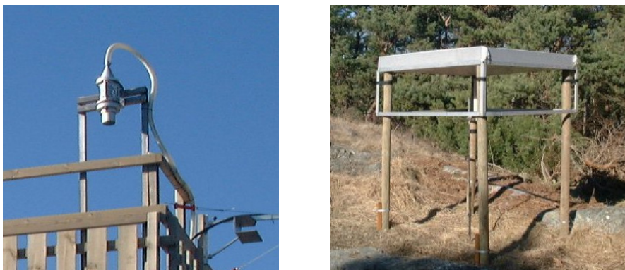
Figure 1. High volume air sampler and deposition sampler.
