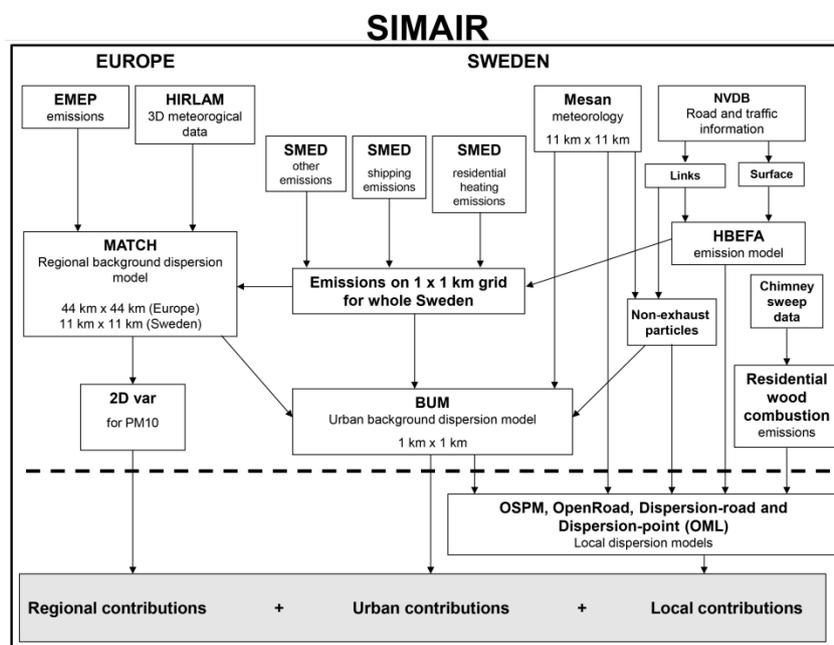
Figure 1. Outline of the databases and models in the SIMAIR system. The dashed line separates stored data and pre-calculated concentrations from larger-scale models (above the dashed line) and concentrations calculated from the web-based user interface (below the dashed line).
