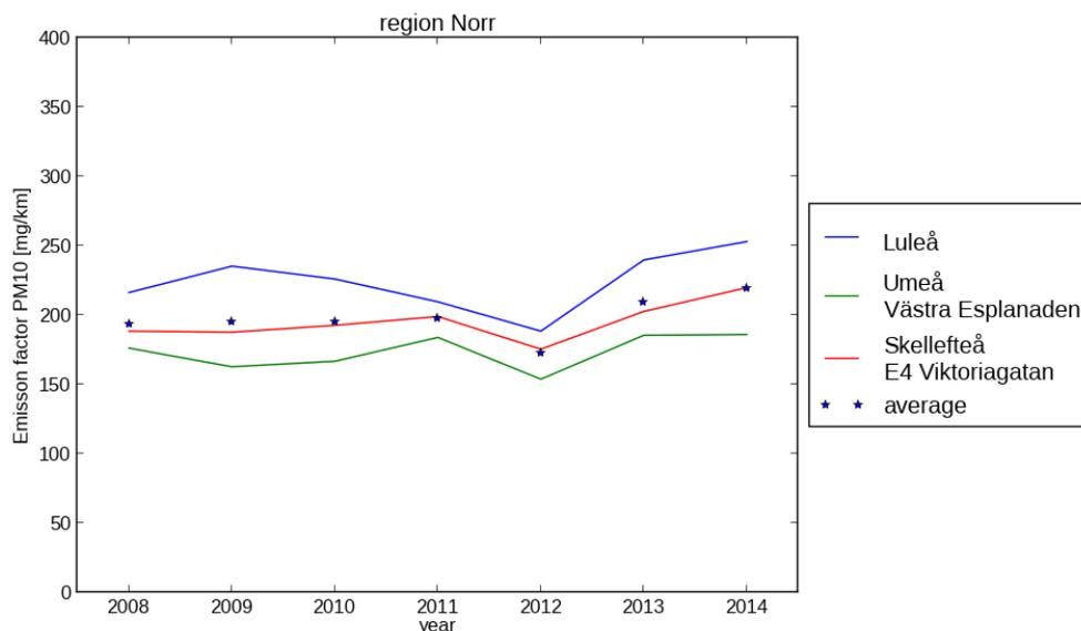
**Figure 2.** Calculated non-exhaust emission factor of PM<sub>10</sub> by SIMAIR for the different streets in region Norr, corrected against monitoring data. In each region, a weighted average is calculated. The non-exhaust emission factor includes both emissions from tyre and brake wear and road abrasion.
