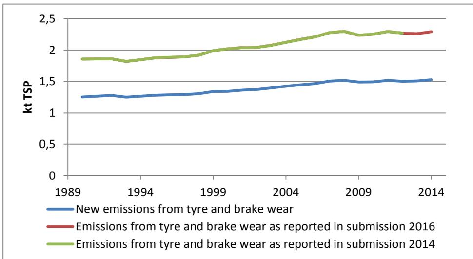
**Figure 18. New TSP emission estimates from tyre and brake wear together with corresponding emissions in submission 2016 and 2014.**
