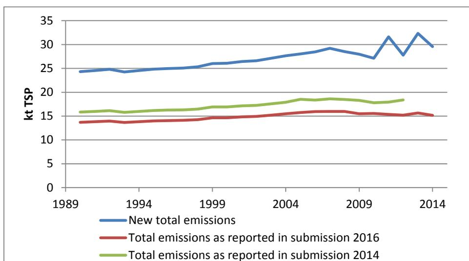
**Figure 13. New total TSP emission estimates together with corresponding emissions in submission 2016 and 2014.**
